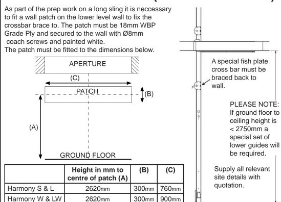
The lower guide brace kit on long slings can accommodate situations where the wall is up to 340mm away from the rear of the aperture. If the distance is greater than this, a special bracing kit will be required.
