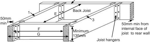
Joist ends should be trimmed onto other joist using proprietary joist hangers or built into structural walls by a min 100mm
