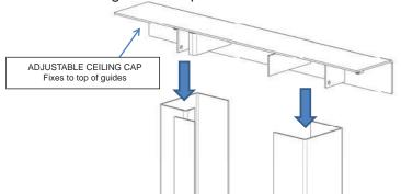
Within each kit are a ceiling plate and ceiling angle. Either one can be used, dependent on the layout of the joists. In all cases a minimum of 4 fixings must be used to secure to joists.
