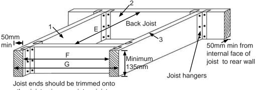
other joist using proprietary joist hangers or built into structural walls by a min 100mm
