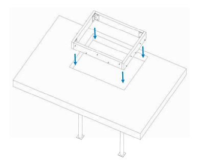
5. ENSURE THE FRAME IS LOCATED CORRECTLY IN THE CUT OUT & POUR THE GROUTING INTO THE GAP FROM ABOVE
