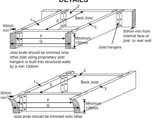
It is essential that the aperture be formed level. Any deviation in excess of 10mm either on the apertures length or width will result in the aperture needing to be re-levelled.
