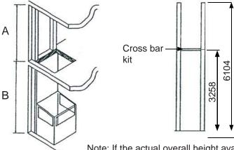
Note: If the actual overall height available exceeds the overall height of the guides (6104mm) then a top guide extension piece (760mm) is required to extend the guides to the ceiling of the upper floor.
