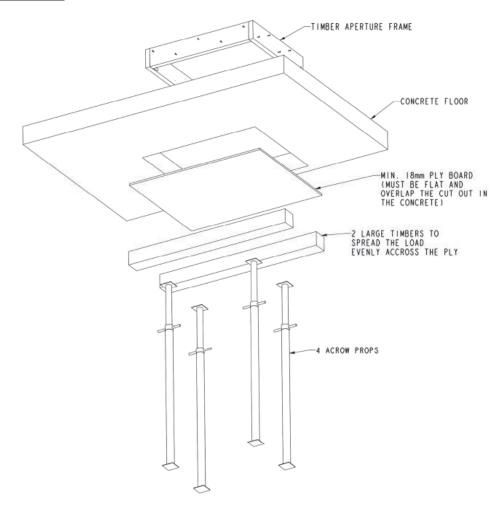
A timber frame needs to be inserted into the concrete floor. When the lift is installed, the steel upper and lower aperture frames for the lift (not shown) will be fitted directly to the timber frame.
