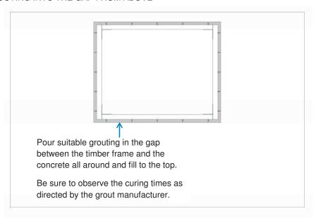
6. WHEN GROUTING IS FULLY CURED, FIX THROUGH THE FRAME INTO THE ORIGINAL CONCRETE FLOOR
