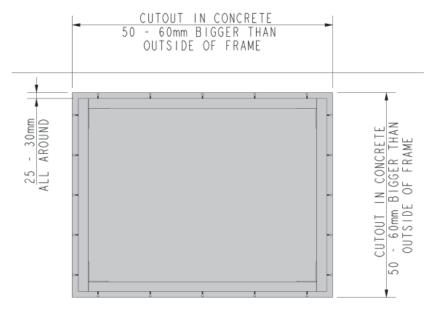
The cut out in the concrete shown in grey also indicates where the timber frame should end up. When the preparation is complete, the gap between the timber and the concrete should be filled with suitable grouting.
