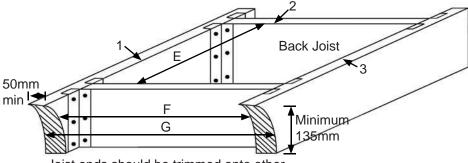
Joist ends should be trimmed onto other joist using proprietary joist hangers or built into structural walls by a min 100mm
